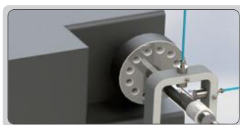
measurement of runout
