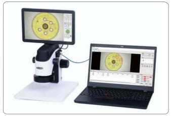
send measurement data and photos to computer, and also take photos, make measurement via computer software
